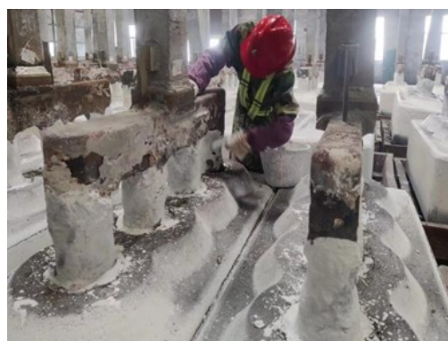
Figure 9. Mixing of coating material in open containers (left) and coating material brushing operation (right).
