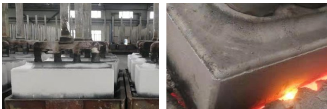
Figure 1. Coated new anode, before enter the cell (left) and during entering the cell (right).
