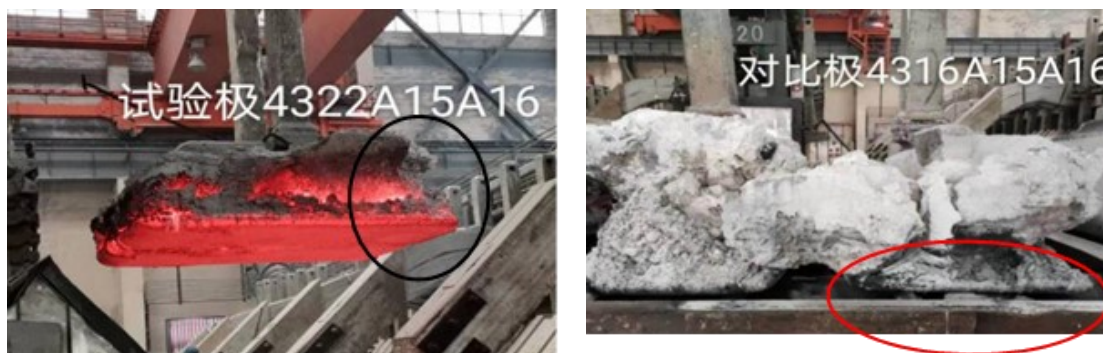
Figure 2. Coated anode butt in test cell (left) and uncoated anode butt in comparison cell (right).
