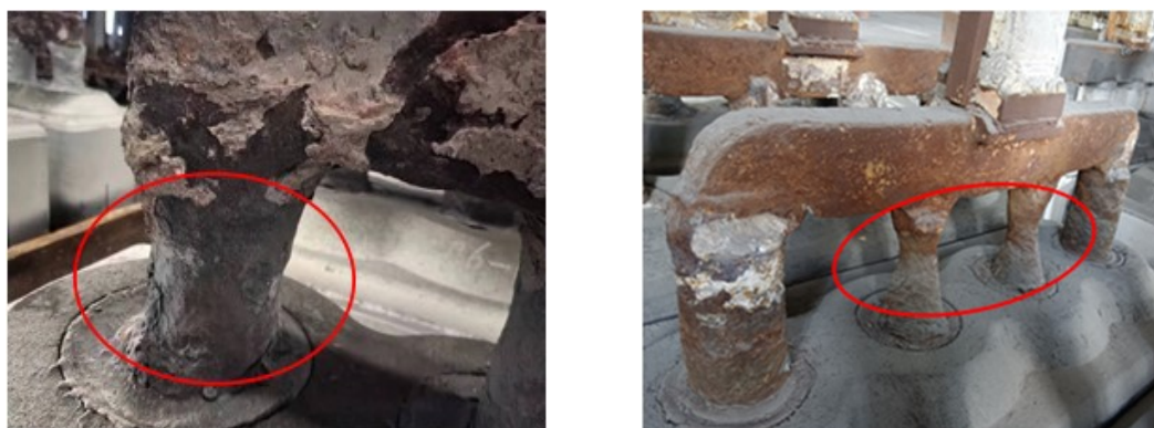
Figure 11. Surface of uncoated stubs (left) and uncoated stubs with “narrow neck” (right).
